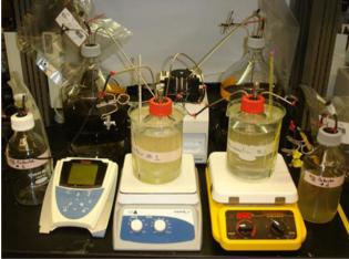
Fig. 1 Schematic (top panel) and photograph (bottom panel) of the experimental apparatus employed in this study. a magnetic stir bar, b stainless steel line, c Viton pump tubing, d gas sampling port, e liquid sampling port. The arrows denote the direction of the liquid flow
